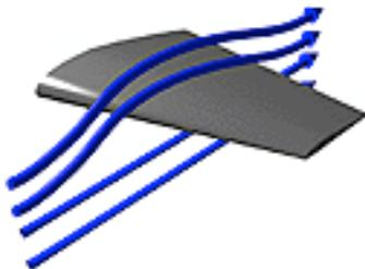
If two particles were released from the same point at the same time, one on each streamline, they would start out moving together. As they approach the front of the airfoil, however, their velocity will start to change. Due to the shape of the airfoil, the air moves faster over the top of the airfoil than it does on the lower surface. The faster air leads to a lower pressure (from Bernoulli's Law) on the upper surface.
