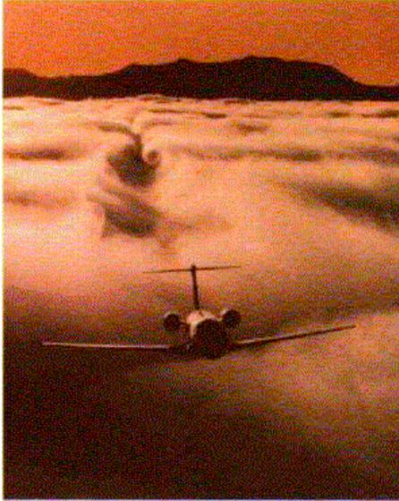
**Fig 6 Downwash and wing vortices in the fog.
