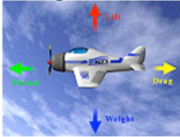
Direction of Forces in Straight and Level Flight
